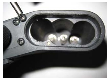
O-ring sealed battery compartment allows use of 2xAAAs or 1x3V Lithium. Your Choice!
